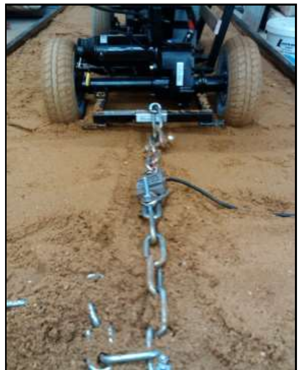
Figure 6: Mobility SF-3713 pulling its own weight to measure maximum force available using the dynamometer load cell and PCE-1000 force gauge
