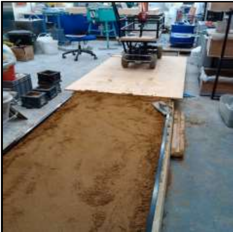
Figure 7: Laboratory experiment sand bed showing acceleration allowance distance (Muleya et al, 2014)
