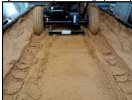
Figure 10: Minimum drawbar-pull generation from the vehicle running on the sand bed terrain at maximum speed with 800N/45PSI.
