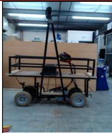
Figure 1: Modified and instrumented Mobility SF-3713 Drawbar-pull laboratory experiments based on MOBILITY SF-3713
